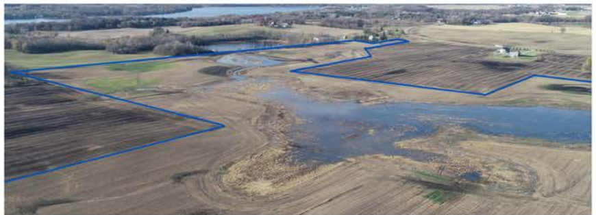
Even with limited rainfall, water levels quickly re-established after the outlet structure was installed in the fall of 2024. BWSR will continue to monitor and manage this site to ensure it is functioning as intended and re-establishes with a diverse mixture of native vegetation.
